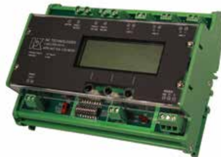
A low profile housing reduces cabinet depth requirements.
